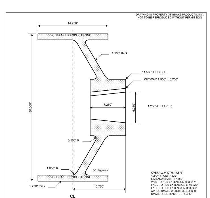
TOLERANCES: WHEEL DIAMETER: +0.005"/-0.000" BORE TAPER: +0.000"/-0.003"
